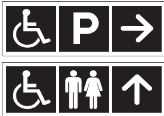
Figure A-3.8.3.1.-A Signs Indicating Accessible Facilities
