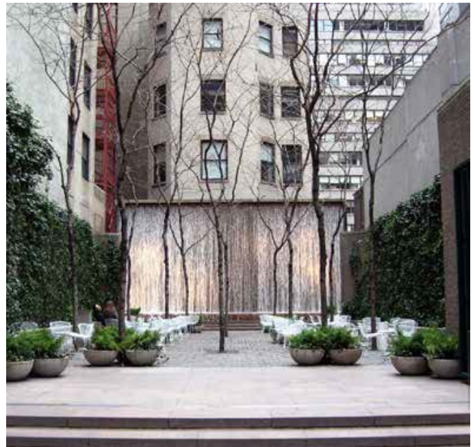
Image | Example of noise mitigation using a pocket park with greenery to create a haven from the busy street front. The water feature generates grey noise, masking surrounding sounds. Paley Park by Zion & Breen Associates, NYC.
