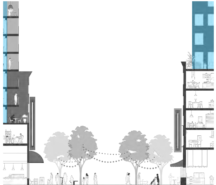
Figure 4: Section | illustrating strategies for balancing active commercial areas with peaceful residential zones, including frontage improvements, noise shielding in mixed-use developments, and social interaction terraces above podiums for quieter, community-focused spaces.
